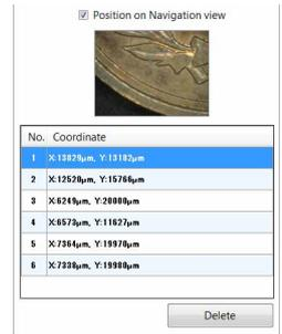
Newly registered coordinates are added to the top of the list. If additional coordinates are registered, when ten coordinates are already registered, the coordinates at the bottom of the list will be deleted.
