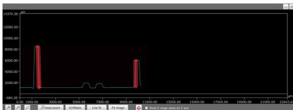
When a measurement interval is set on a profile, the measured value appears in the profile display area and in the profile/measurement list.
