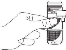
**2 Place a white object on the stage and focus on the object.**
