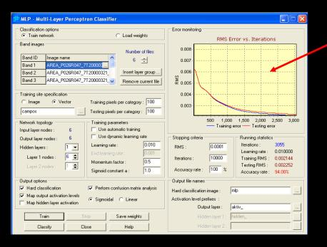
Red and blue lines should be in close alignment. Both lines should slope down in time.
